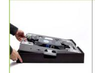
Each LED tile is packed in a shock absorbing foam protector, to prevent any damage to the LEDs or LED panel during transport.
