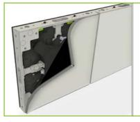
LEDskin® frames can easily be finished at the back using textile or panels (patented design), which can be easily attached using silicon edges or hook and loop tape.
