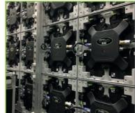
The tiles are aligned using magnets, whilst two manual connectors ensure a strong connection.
