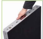
For optimal handling we kept all LED panels as light as possible. Integrated grips and handles are provided.
