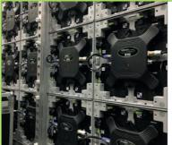
The tiles are aligned using magnets, whilst two manual connectors ensure a strong connection.
