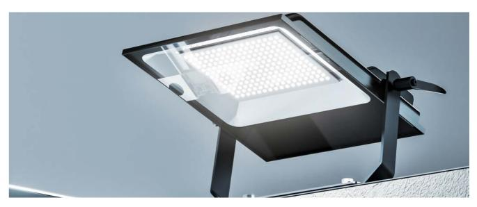
ART. NR: 250 05 63 10X DIMENSION: 475X490X550 MM WEIGHT: 5 KG LUMINOUS FLUX: 23 000 LM ELECTRICITY CONSUMPTION: 200 W BEAM ANGLE: 120° COLOUR TEMPERATURE: 3000 K / 5000 K COLOUR: BLACK CONTENT OF 1 BOX: 10 BIG LIGHTS, 10 BRACKETS, 2 POWER SUPPLY CABLES OF 1.5 M, 10 LOOP-THROUGH CABLES OF 3 M
